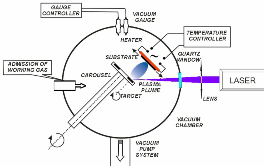
Fig.1. General schematic of the PLD setup used in experiments
