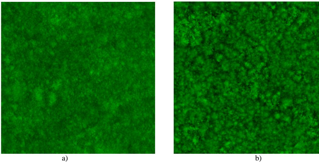
Fig. 4. Surface topography, zoom 1, 10 X magnification, for a) 6P57 and b) 6P61 bioglass films.
