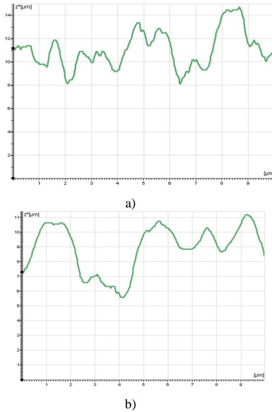
Fig. 3. Surface profile along a random 10  $\mu\text{m}$  length zone in the cases of a) 6P57 and b) 6P61 bioglass films on Ti substrates.
