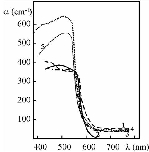
Fig. 15. Dependence of the absorption coefficient on wavelength for the glasses of the system  $\text{Ge}_{20}\text{As}_{14}(\text{S}_{0.5}\text{Se}_{0.5})_{66-x}\text{I}_x$ , for: 1)  $x = 0$ ; 2)  $x = 2$ ; 3)  $x = 6$ ; 4)  $x = 10$ ; 5)  $x = 14$ .
