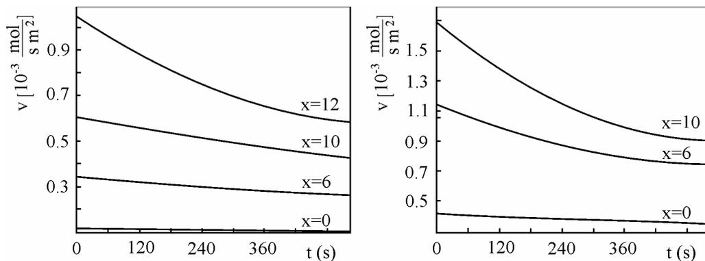
Fig. 7. Rate of dissolution of glasses of the system  $\text{Ge}_{20}\text{As}_{14}(\text{S}_{0.5}\text{Se}_{0.5})_{66-x}\text{I}_x$  as a function of time a) in 2 [mol/dm<sup>3</sup>] KOH; b) in 5 [mol/dm<sup>3</sup>] KOH.
