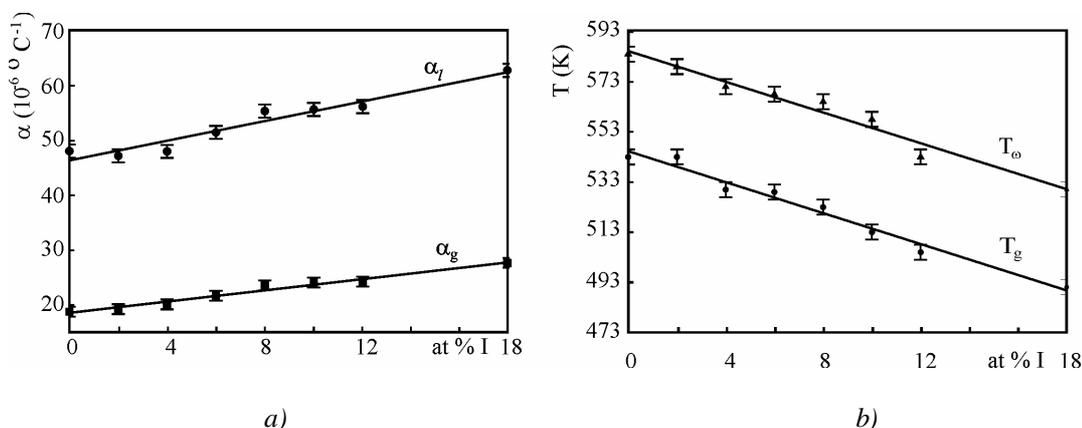
Fig. 13. Dependence of thermal coefficient of linear expansion (a) and of  $T_g$  and  $T_\omega$  (b) of the glass  $\text{Ge}_{20}\text{As}_{14}(\text{S}_{0.5}\text{Se}_{0.5})_{66-x}\text{I}_x$  on iodine content.
