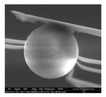
Fig. 1b. SEM pictures of attached spheres with a 25  $\mu$ m diameter.
