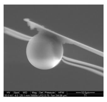
Fig. 1a. SEM pictures of attached spheres with a 20 µm diameter.
