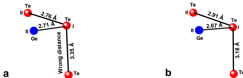
Fig. 3. a. RMC model E_{total/atom}=4.7*10^5 dynÅ Ge coordination: 2.53 Å, 2.71 Å, 2.74 Å, 2.63 Å b. RMC + Lennard Jones relaxation : 17 500 iterations; E_{total/atom}=2.3*10^5 dynÅ; Ge coordination: 2.53 Å, 2.67 Å, 2.76 Å, 2.63 Å
