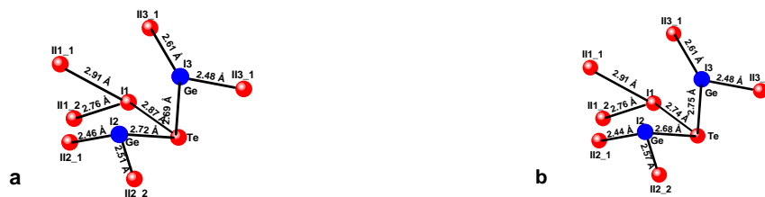
Fig. 4. Two local configurations in the Ge-Te model: a. RMC model E_{total/atom}=0.67*10^{-5} \text{ dyn}\text{\AA} b. RMC + after relaxation with Lennard-Jones potential: 17500 iterations; E_{total/atom}=0.606*10^{-5} \text{ dyn}\text{\AA}
