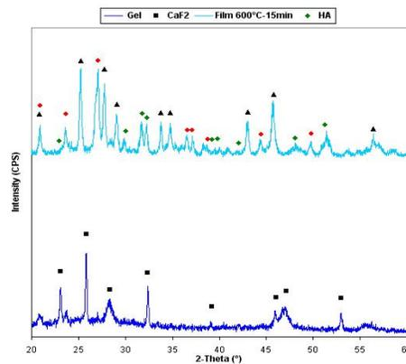
Fig. 1. XRD patterns of the first chemical route: gel and HA/FA film heat-treated at 600 °C for 15 minutes.
