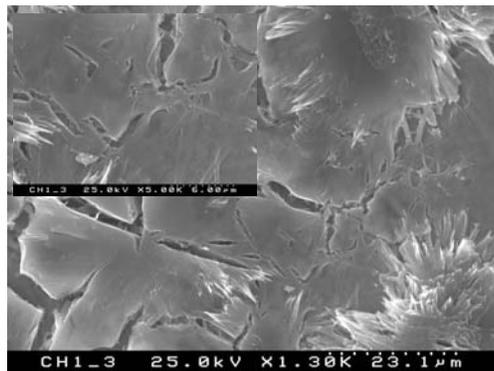
Fig. 2. Scanning electron microscopy photos of FHA 1 layers on Ti6Al4V annealed at 600 °C for 15 minutes in air, withdrawal speed of 0.5 mm/s.
