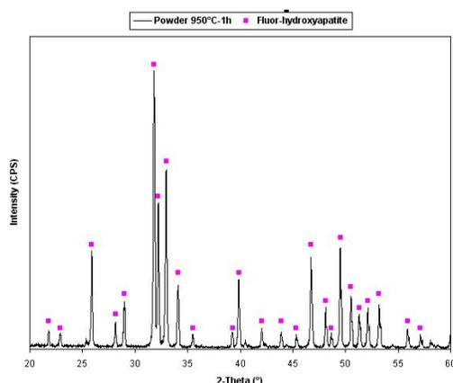
Fig. 3. XRD patterns of third route fluor-hydroxyapatite powder calcinated in air at 950°C.
