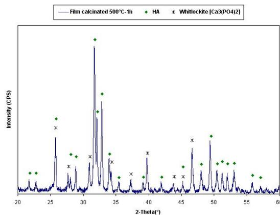
Fig. 1. XRD patterns of the second route fluor-hydroxyapatite thin layers onto Ti6Al4V.
