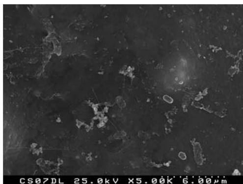
Fig. 3. Scanning electron microscopy photos of a 21 days immersed Ti6Al4V coated sample in simulated body fluid.
