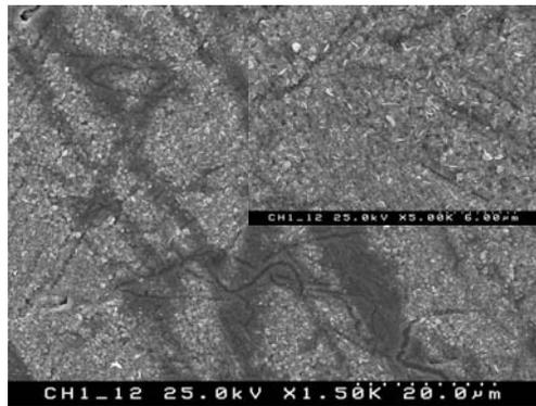
Fig. 2. Scanning electron microscopy images of a Ti6Al4V dip coated sample at a withdrawal a speed of 1.2 mm/s.
