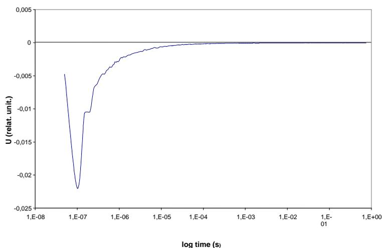
Fig. 3. The electric signal measured on *Leptosphaeria rhodopsin* oriented sample. Measuring conditions were 100 mM NaCl, 50 mM MES, pH 6, and 20°C.
