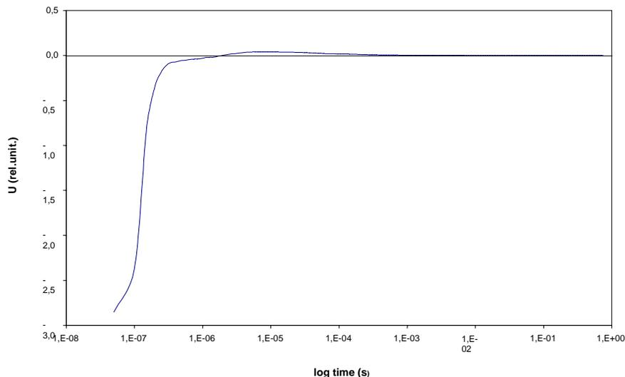
Fig. 2. The electric signal measured on bacteriorhodopsin oriented sample. Measuring conditions were 100 mM NaCl, 50 mM MES, pH 6, and 20°C.
